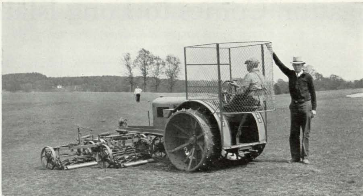
TORO TRACTOR WITH WIRE CAGE ENCLOSURE FOR THE OPERATOR This device is used by George Post, greenkeeper at Franconia Club, Springfield, Mass.
