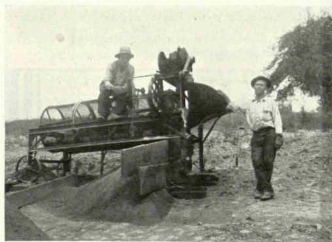
ROTARY SCREEN USED AT CHARTIERS HEIGHTS Notice how fine the soil is. This was used for topdressing fairways
