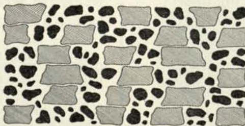
Plate No. 3—Shows Earth with Humus Particles Dry and Contracted.
