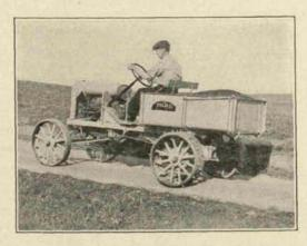
general utility, hauling around the course, grading and construction work, together with numerous other drawbar needs. In addition, it can be equipped with three standard 30-inch mowers, either in front,—similar to the regular golf machine,—or behind, in conjunction with a pull frame.
