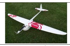
Aeromao Aeromapper fixed-wing UAS. Image courtesy of Aeromao.com.
