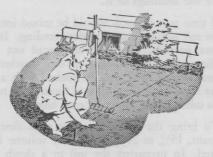
Certain points must govern the grading, including the elevation of the house, sidewalk or curb and trees. The grade between these fixed points should be pleasing to the eye and sloped sufficiently to permit adequate surface drainage. Depressions in which water will stand and ice form should be avoided, as either condition is injurious to grass.
