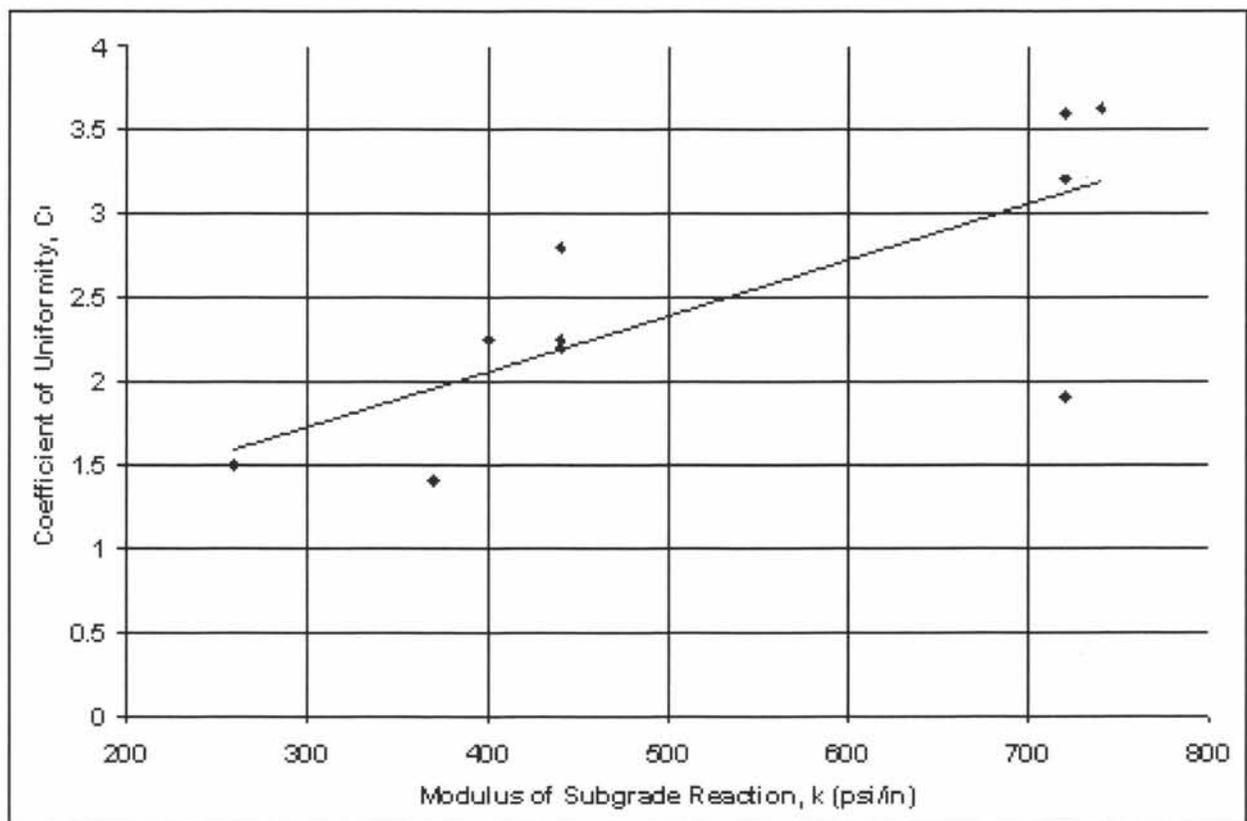
Figure 5: Coefficient of Uniformity and Modulus of Subgrade Reaction
