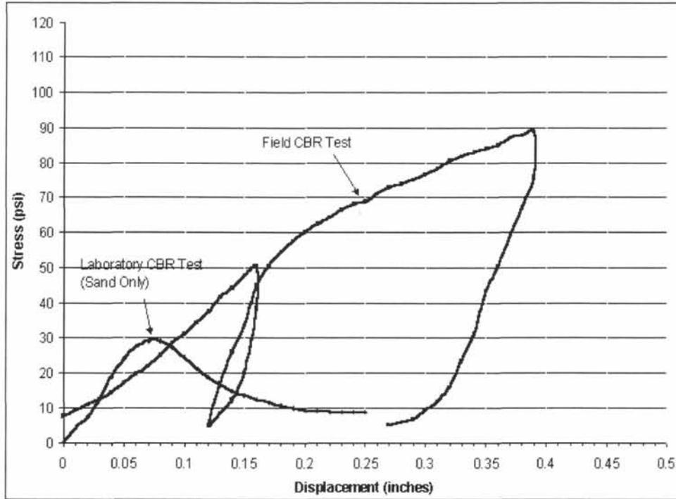
Figure 7: Laboratory and Field CBR Tests
