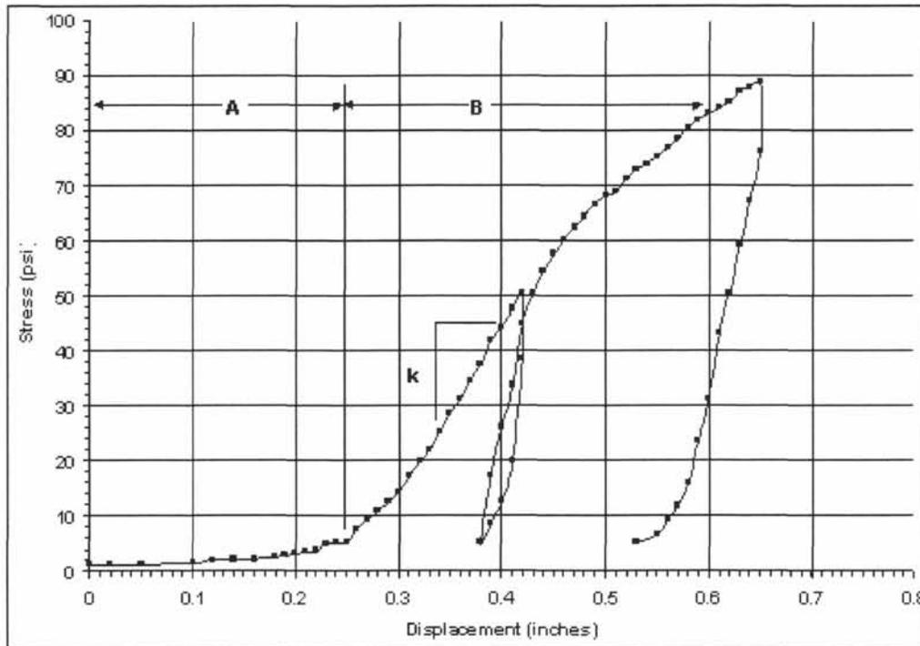
Figure 4: Field CBR Test Results
