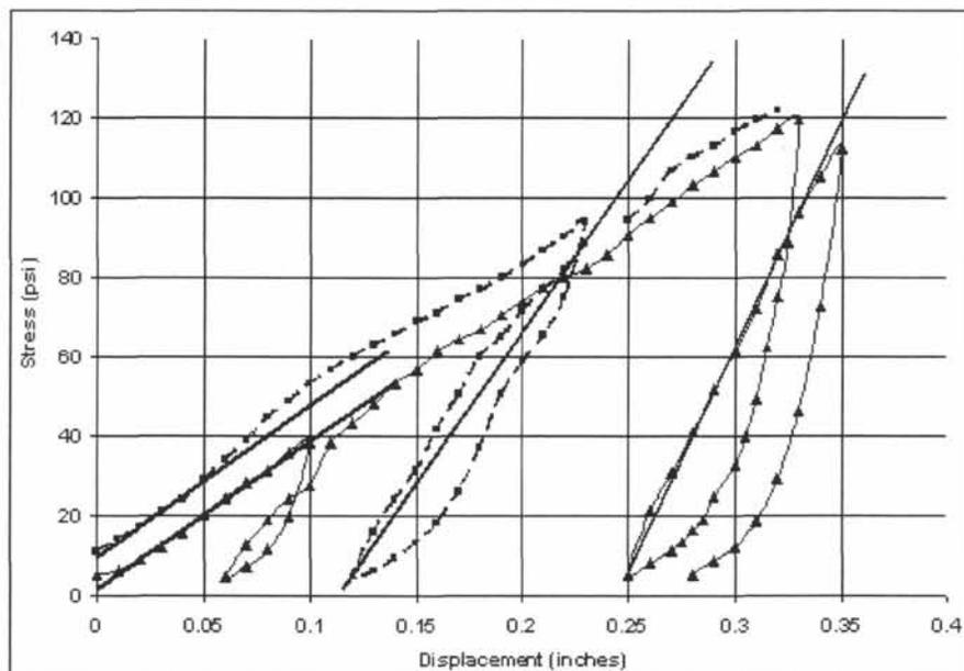
Figure 8: Stiffness as a Function of Time. Three Month Time Between Tests on Same GreenFindings
