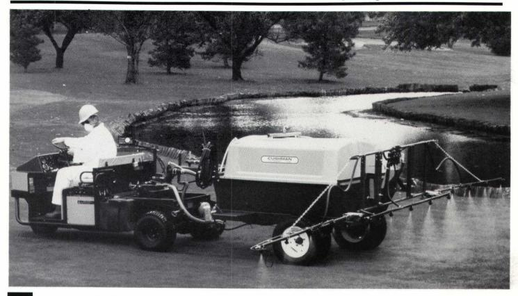
his Cushman<sup>®</sup> 5th Wheel Sprayer gives you the best of both worlds--high capacity to reduce timeconsuming refills and low psi to keep ground pressure to a minimum. The tank is configured to distribute the weight across both implement and Turf-Truckster<sup>®</sup> tires. The result is an incredibly low 11 psi ground pressure to help protect fine turf.
