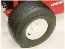
Larger floatation tires not only minimize compaction, they also make the machine easy to control.
