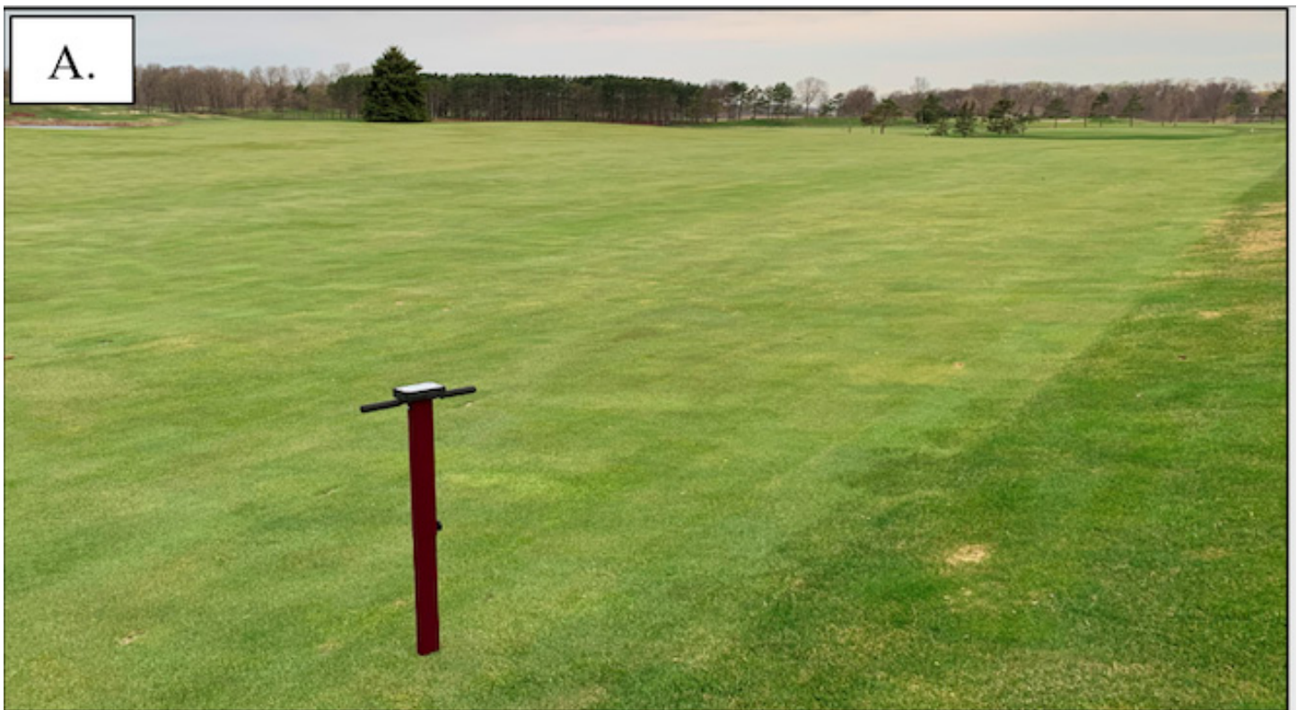
Figure 1 A. Data collection and soil moisture map creation process: A) a FieldScout TDR 350 collecting and georeferencing (i.e. recording latitude and longitude location) soil moisture data from a fairway
