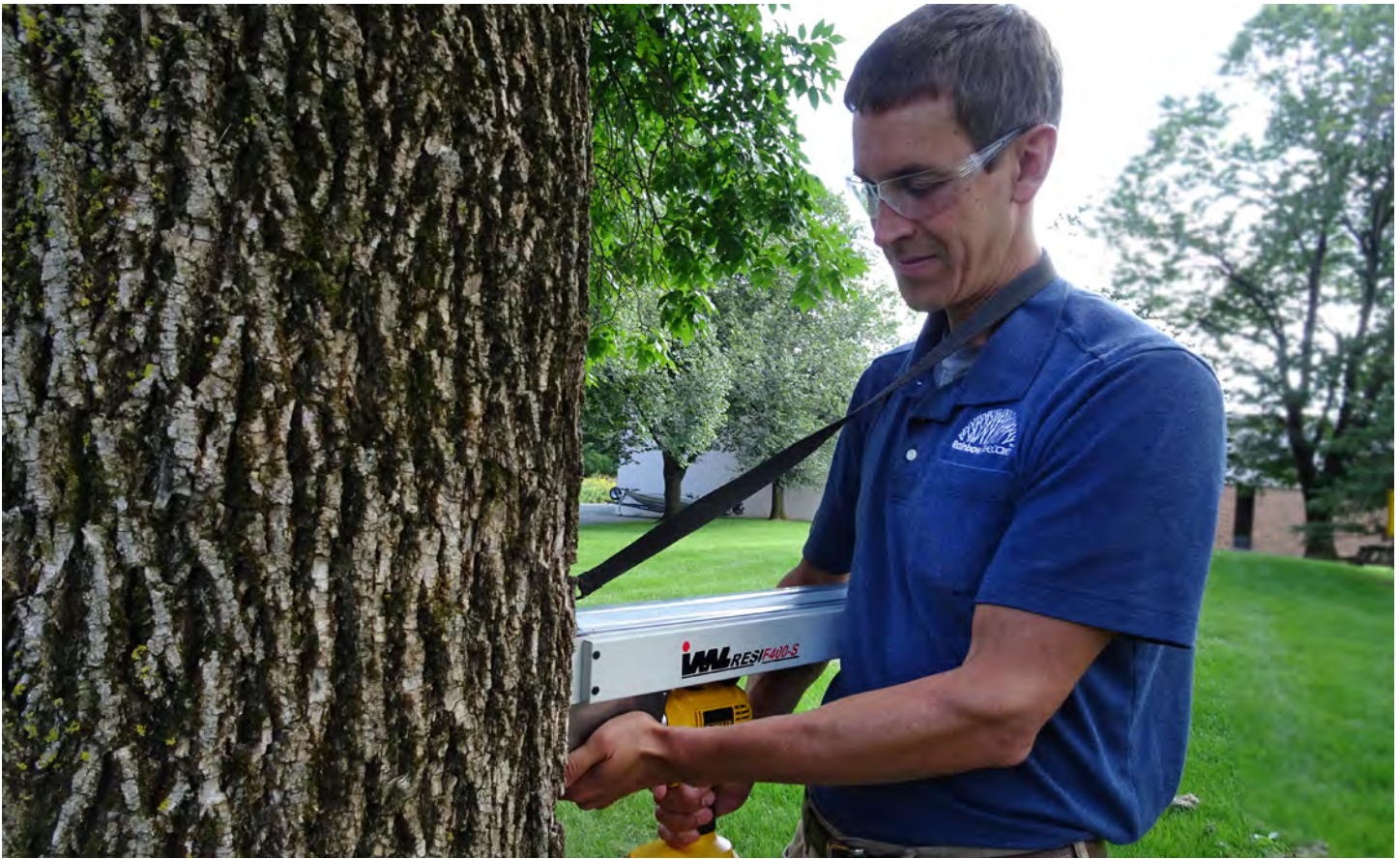
An arborist demonstrates a resistograph
