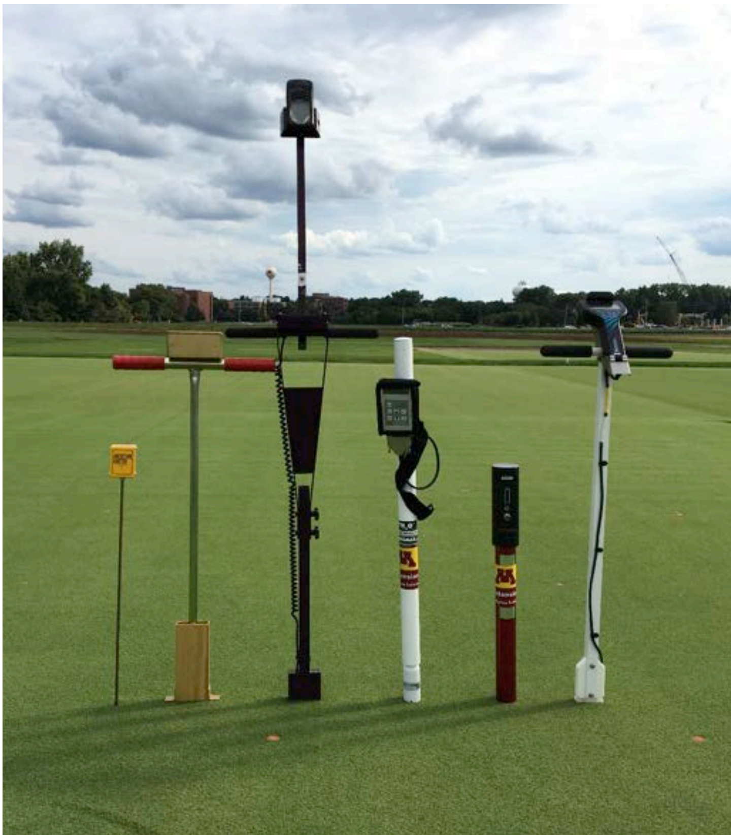
Image 1: A variety of portable soil moisture meters. From left to right- Spectrum Economy Soil Moisture Tester, Turf-Tec Digital Moisture Sensor, Spectrum FieldScout TDR 300 w/ GPS, Delta-T TH2O Soil Moisture Meter, Stevens Water POGO, Campbell Scientific Hydrosense II
