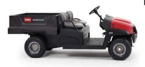
The Workman GTX is adaptable for any task. Two or four-seat configurations come with bench or bucket seats. Front and rear attachment points for garbage cans, hose reels or walk spreaders free up the bed for more hauling capacity. 4 and 6-foot flat beds are also available.
