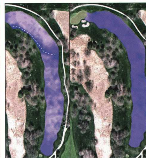
Figure 7. Drainage. The left picture shows soil moisture levels before installation of drainage with after drainage soil moisture levels on the right. The dotted line represents the drain tile installation. The darker the blue the higher the soil moisture.
