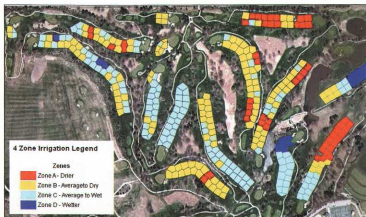
Figure 4. Map of Irrigation Management Zones. Irrigation programming based upon this concept can conserve water and reduce pumping costs.
