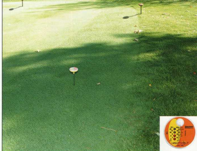
Figure 5: LightScout sensors placed on and around a golf green to collect daily light levels. (Scott Lemke)
