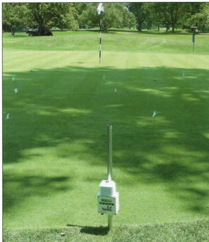
Figure 4: Mini weather station positioned on the side of a golf green for collecting daily light levels. (Derek Settle, CDGA)
