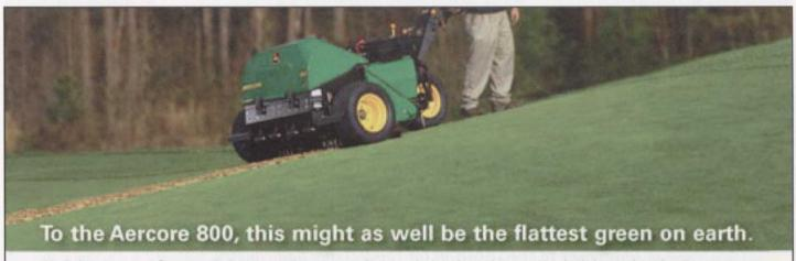
It's all the same to us. Because whether a green has a severe slope, rolls a little bit, or has no roll at all, our Aercore\* 800 Walk-Behind Aerator can produce an even depth of coring on all of them. Unlike some walk-behind aerators that position the coring heads behind the wheels, the Aercore 800 has its coring head between the wheels. This allows the coring head to stay at a consistent level to the ground.
