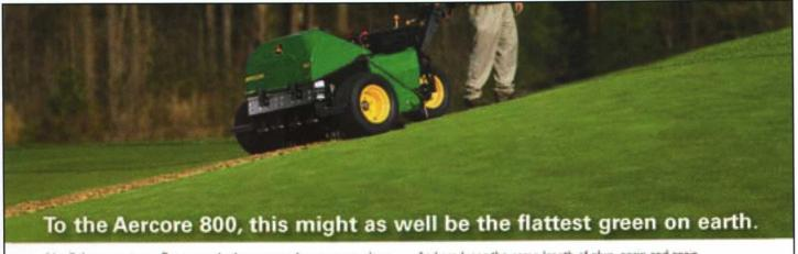
It's all the same to us. Because whether a green has a severe slope, rolls a little bit, or has no roll at all, our Aercore<sup>22</sup> 800. Walk-Behind Aerator can produce an even depth of coring on all of them. Unlike some walk-behind aerators that position the coring heads behind the wheels, the Aercore 800 has its coring head between the wheels. This allows the coring head to stay at a consistent level to the ground.
