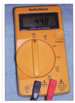
To sum things up, you need to get a meter that is durable, digital and does at least AC voltage and resistance (ohms). Attached leads are nice, and you want to
