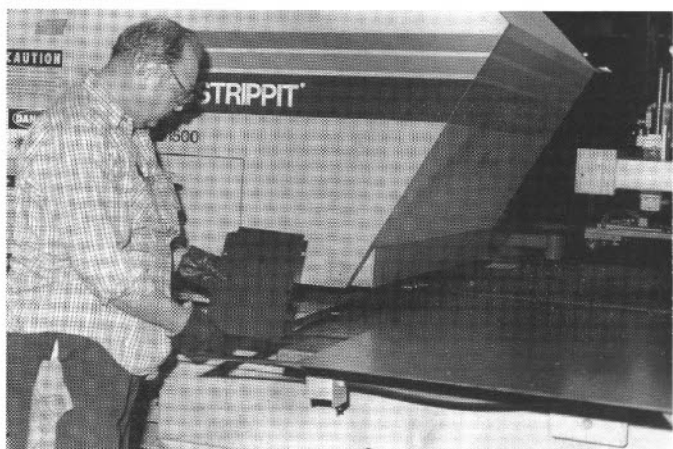
Jacobsen uses a laser cutter to cut sheet metal parts. The laser cutter operates off programs developed by the company's CAD/CAM system, and provides fast, simple, uniform cutting for such parts as couplings, necks, fenders, and other sheet metal parts.
