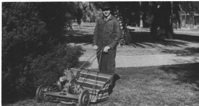
Jacobsen's 4-Acre Mower, introduced in 1921, was the first mower equipped with a gasoline engine specifically tailored to power mower specifications.
