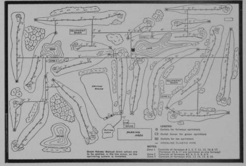
This is a typical layout (greatly reduced) of the kind of plastic pipe sprinkler system plan we develop for an individual course. It is part of the CRESline Engineering Service that has helped hundreds of golf clubs install efficient, economical sprinkler systems.
