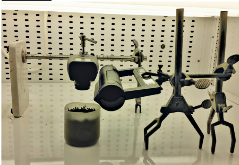
Time-lapse photography was used to capture annual bluegrass weevil (ABW) surface movement in growth chamber studies. Weevils were marked with a UV pen and placed in groups of five on a Poa annua plug. The black light illuminated the mark during dark periods.
