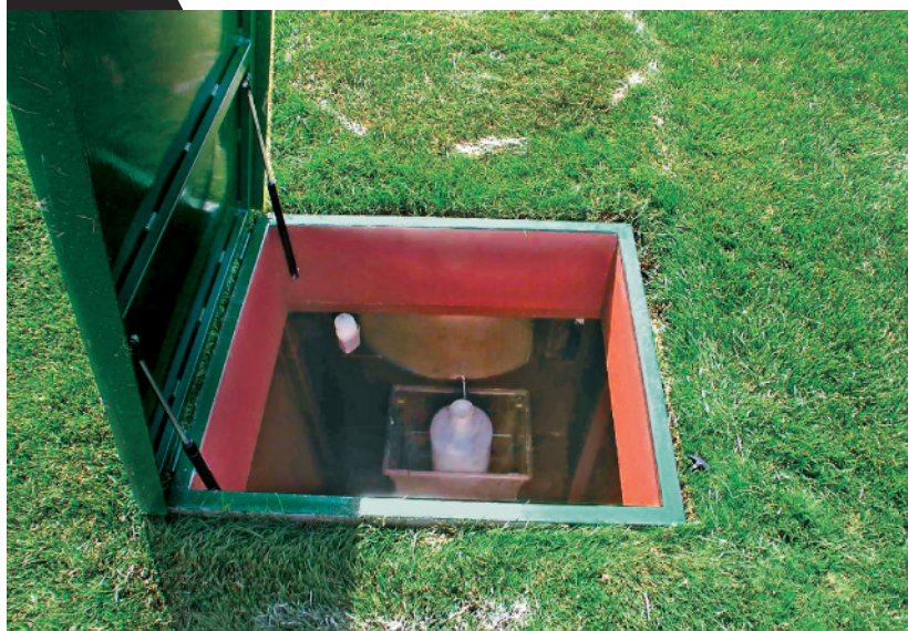
The bottom portion of the stainless steel lysimeter and the carboy that collects leachate can be seen inside the access chamber.
