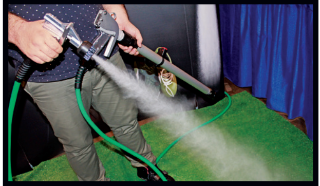
The Zeblaster propels extremely fine droplets of water at .06 gallons to .26 gallons of water per minute.
