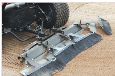
Smithco Exclusive: Tournament Series Rake with Flex-Brush – Eliminates unsightly “doughnuts.”
