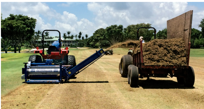
Anderson and his staff used the Koro Field Top Maker to complete the fraze mowing process on Card Sound GC's fairways, while Wheeler fraze mowed half of Wycliffe G&CC's practice range tee.
