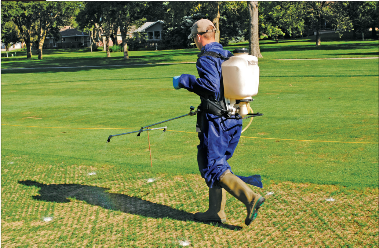
A backpack boom sprayer is easy to make accurate, and can be used to apply pesticides uniformly to small areas and/or around obstacles.
