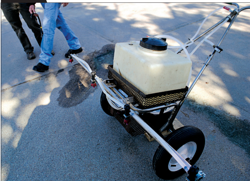
An 8-gallon boom sprayer fabricated on a rotary spreader frame at Lochland CC in Hastings, Neb., by Craig Ferguson and his staff.
