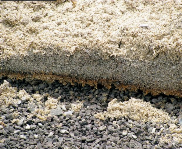
Iron layer at sand/gravel interface (12-inch depth) of Hawaii putting green. The layer reduced water infiltration, resulting in anaerobic soil conditions and thin turf density at the surface.
