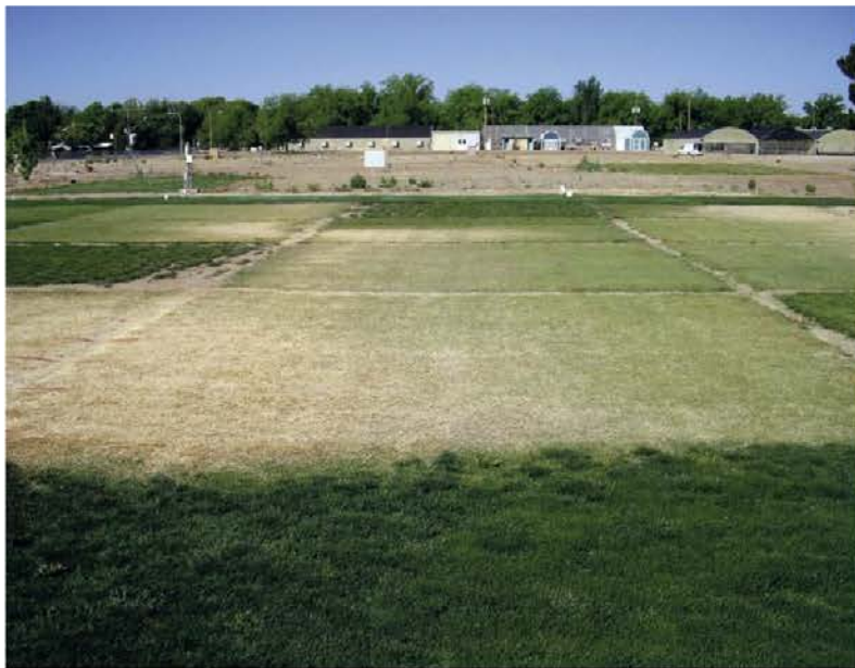
Right side of the image is the irrigation source (linear gradient irrigation system). Amount of applied water goes from none on left to 150 percent ET on right. You can see the four turfgrass species as you progress away from the camera.
