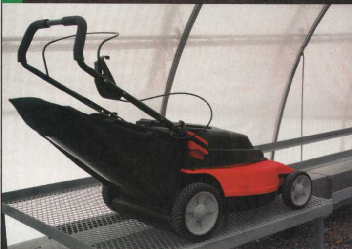
A cordless lawn mower traverses the bench and mows potted turf. Clippings are collected in a bag made of quarter-inch hardware cloth.
