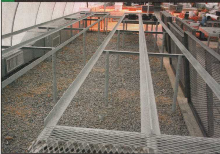
Adjustable metal racks hold potted turfgrass beneath angle-iron tracks.
