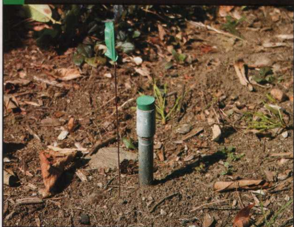
Suction lysimeter inserted in soil to a depth of 20 inches. Rubber stopper at top is removed to evacuate the lysimeter tube and withdraw soil water sample.
