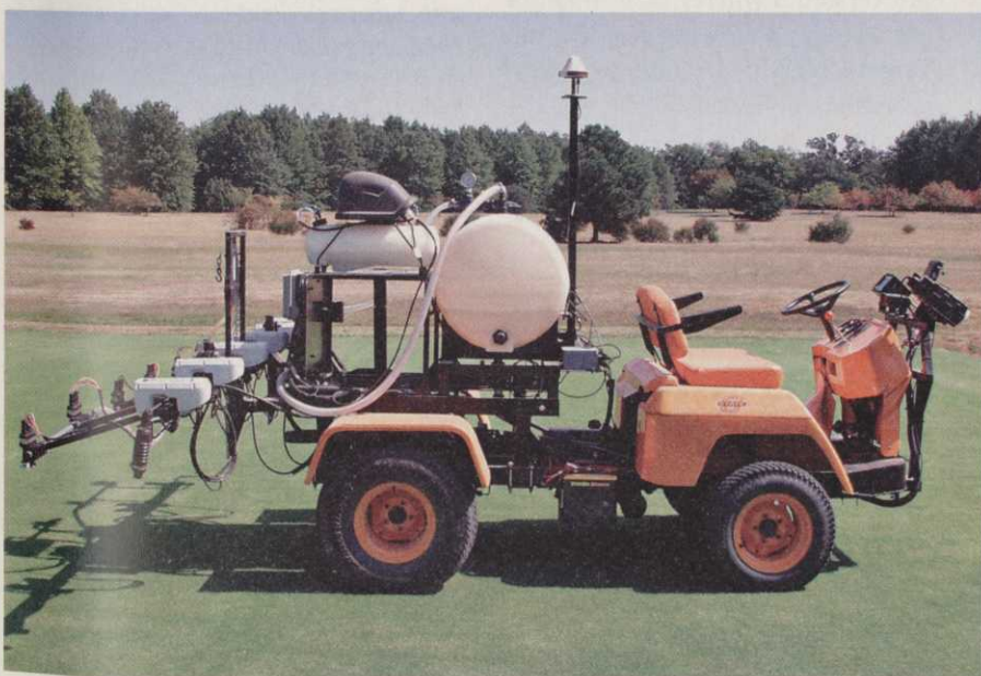
Sensors may be used with a variable rate nitrogen applicator (shown here) to maintain healthy turf by applying prescribed rates in areas as small as 2 square feet.
