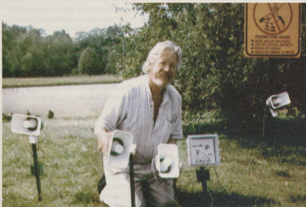
The Alarm/Alert Goosebuster call playback successfully disperses geese and prevents re-colonization of areas.
