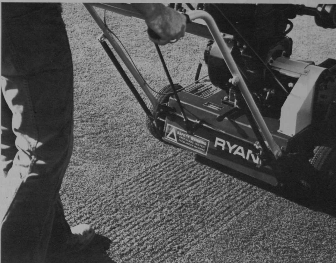
Vertical cutting blades can be seen underneath the verticutting machine at left. Effect of verticutting on turf is shown above.
