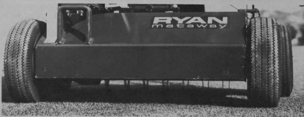
Vertical cutting blades can be seen underneath the verticutting machine at left. Effect of verticutting on turf is shown above.
