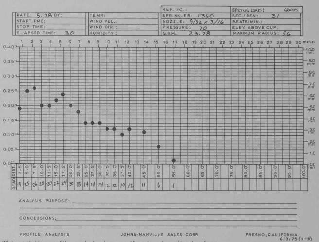
This sprinkler profile analysis shows uniformity of application for a particular sprinkler under a given set of conditions.
