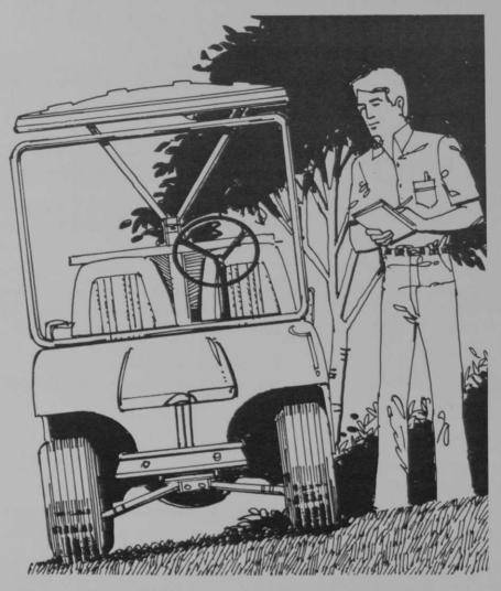
time to look for cracks in the fiberglass or dents in the metal - though it's best if the car is inspected for these things after each rental. Either way, if damage is found which might affect the structural integrity of the body or interfere with movement of the wheels or suspension, pull the car out of service to be repaired.
