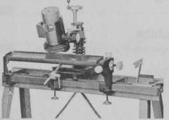
Foley's Bed Knife Grinder Foley's Bed Knife Grinder provides exact angles for precision sharpening. Grinds bed knives and straight knives up to 36" long.
