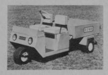
tive steering. The GT-7 features double seats with back rests, 950 by 86-ply Terra-Tires, dump body (corrosive resistant), trailer hitch, dual headlights, 35 amp alternator, ammeter, oil pressure indicator, speedometer, heavy-duty shock absorbers, automotive hydraulic internal expanding brakes, and an 18hp Onan engine. Suggested retail: \$1,788.
