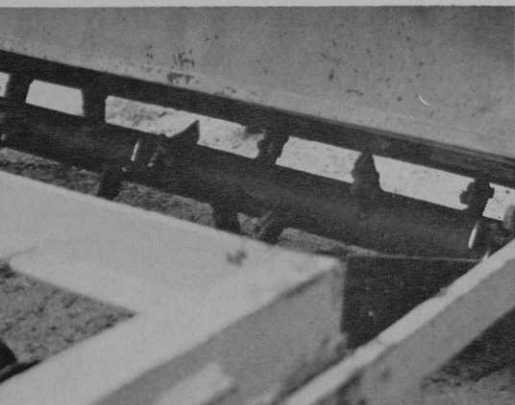
(Left) Here is a closeup of the front shaft, with knives which loosen the soil. At right, is overall view of the planter with cultivating knives in front, two rows of cutting discs in center, and roller behind.
