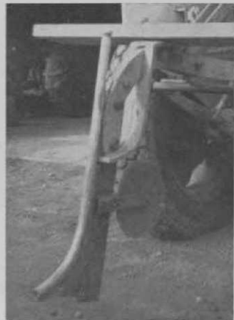
The Haines root pruner as modified for laying underground cable.
