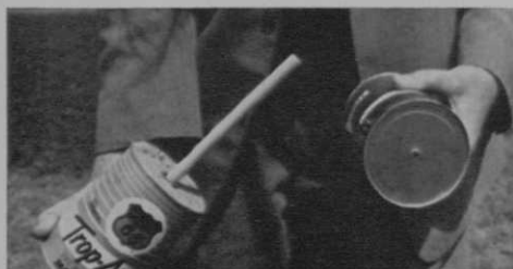
Plot marker made from a used quart size oil can. The drainage hole is shown at the right, pipe and stake at left.
