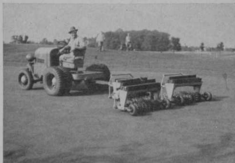
At Detroit's Maple Lane, weights on 3-gang spiker are old railroad rails.
