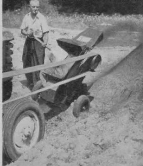
Royer Model M-2 (up to 8 cu. yds. per hour) at York Downs Golf Club, Toronto, Canada.
