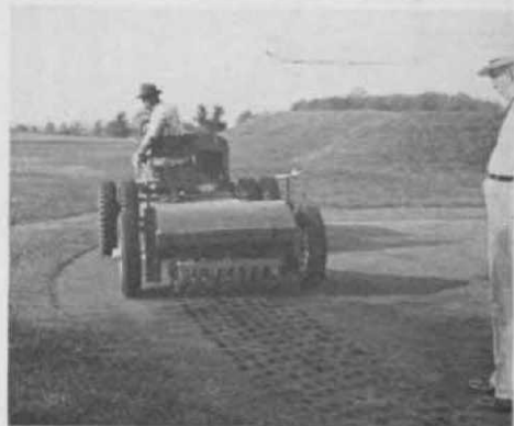
Aerifier on green, showing raised turf around each hole. Rolling lightly in opposite direction following removal of plugs puts green in shape for immediate play.
