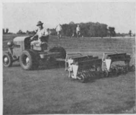
Three gang spike discer on green. This tool helps prevent dry spots. Makes greens take water better but is ineffectual after dry spots develop.
