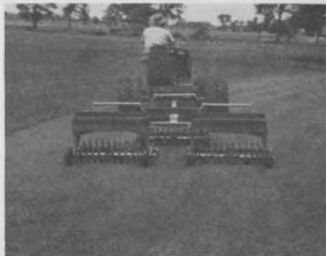
Frequent use of three-gang spiker on greens at Maple Lane CC, Detroit, keeps them in top shape with minimum of water.
