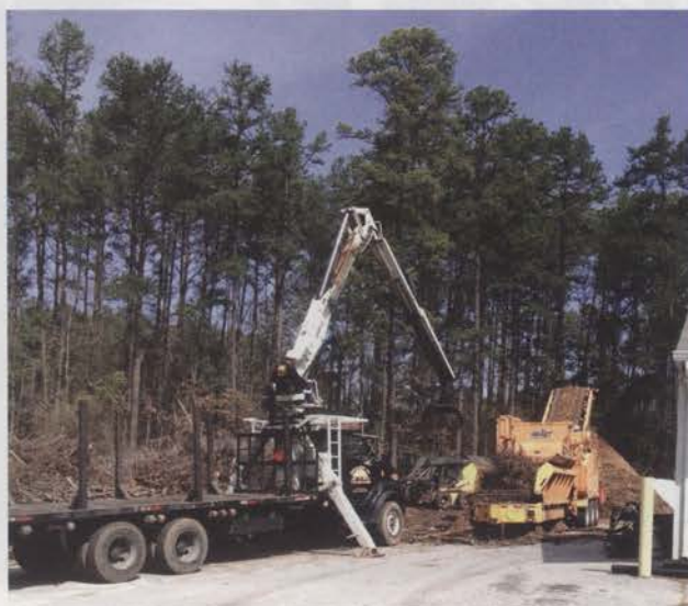
Large or small grinding equipment can turn organic wastes into useful mulch and save money on landfill and disposal fees.
