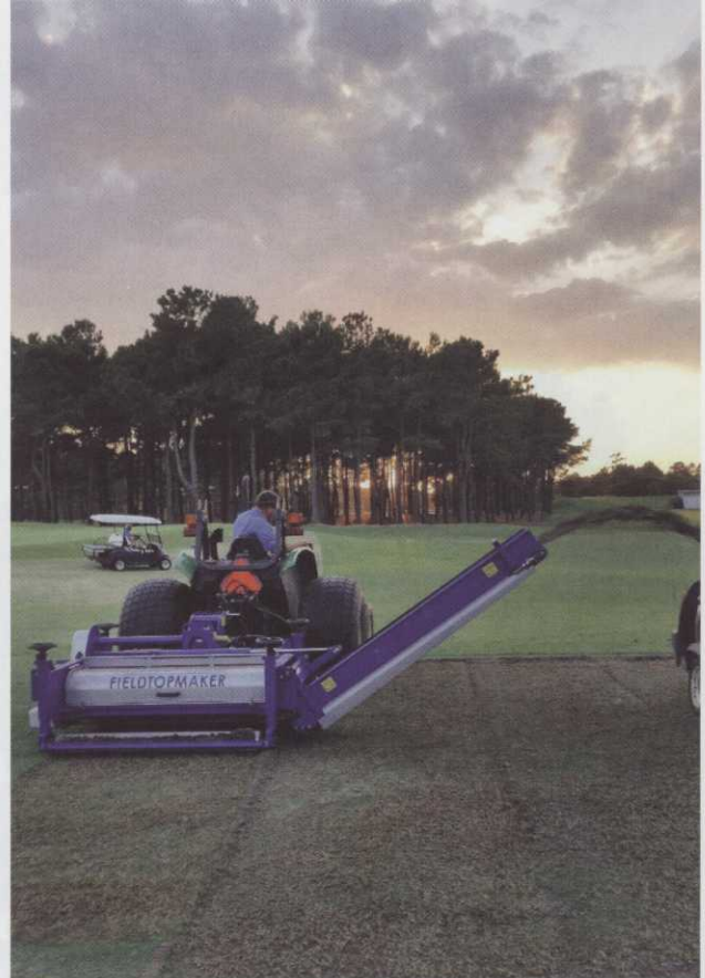
Fraze mowing, which aggressively removes the top layer of turf, has entered the North American golf market. Above: the technique being used on an approach.
