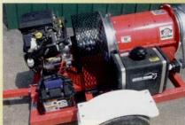
Gator. The engine battery is used to change the blower nozzle direction, as it is hooked up to the alternator on the tow vehicle with pig tails to keep the battery charged at all times. The blower RPM's are changed as needed by changing the ground speed of the tow vehicle with the throttle lock when desired. The blower is significantly quieter than when it had an engine and it saved the club over \$2,000 for a new engine. The used real motor cost \$65 and it took about eight hours to build.
