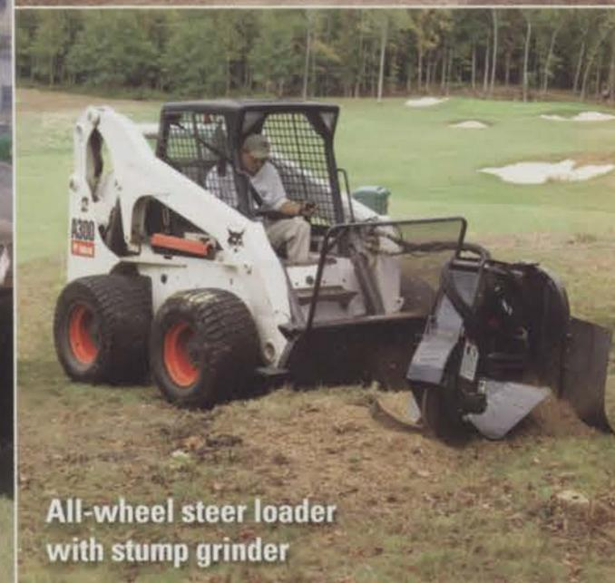
All-wheel steer loader with stump grinder
