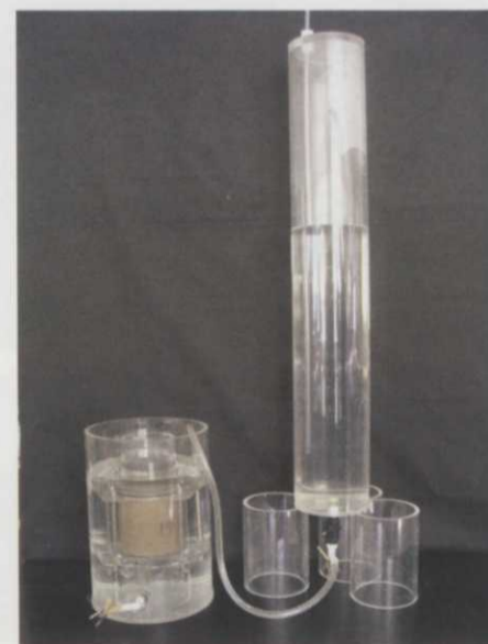
The saturation tank and permeameter was combined into a single system.
