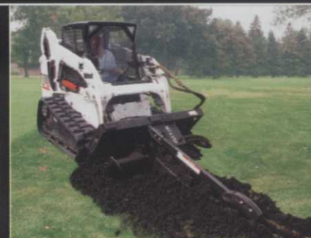
Track loader trenching irrigation line
